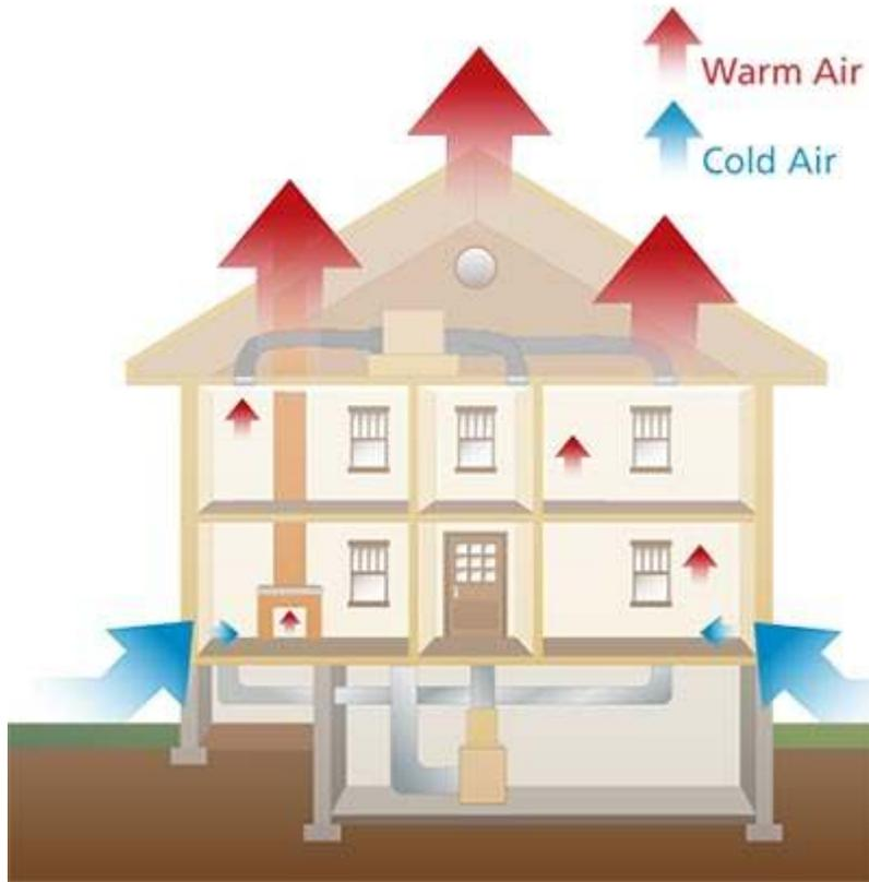
**Stack ventilation is greatly predictable and preferred over cross ventilation because the former takes advantage of natural buoyancy and is not dependent on direction of wind flow.**
